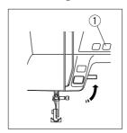
Raise the presser foot. Press the needle up/down button ① to raise the thread take-up lever to its highest position.
