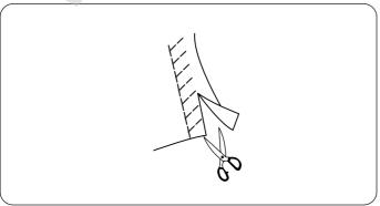
Place your fabric to allow a  $5/8^{\prime\prime}$  (1.5 cm) seam. Trim excess close to stitching. Be careful not to cut the stitches.
