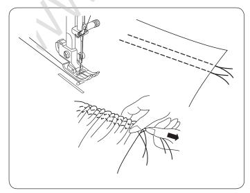
Loosen the thread tension to "1" and increase the stitch length to 5.0.
