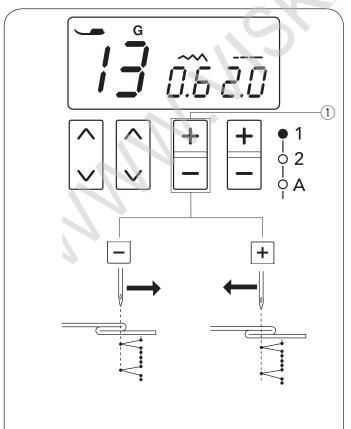
Adjust the needle drop position as follows:
